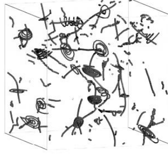
Fig. 2: Axes of elementary vortices and streamlines relative to the axes in a freely decaying turbulence. [1]
