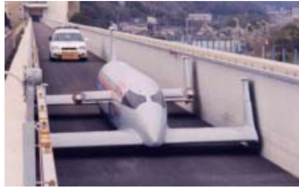
Fig.2 Running test using the second phase model ART002 ( V=120\text{km/h} , W=400\text{kg} )
