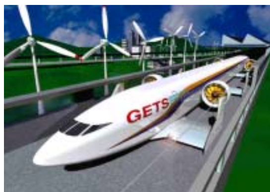
Fig.1 Image sketch of the Aero-Train (3 cars, V=500\text{km/h} )
