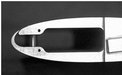
Fig. 3. The NACA 0015 airfoil model with blowing slot (Ref. 5)
