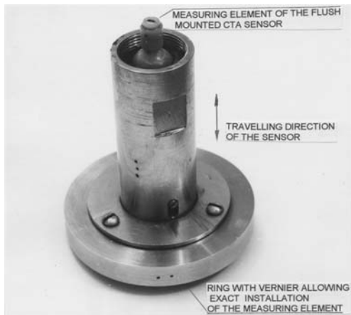
Fig. 2: Device to clamp flush mounted 55R46 CTA sensor
