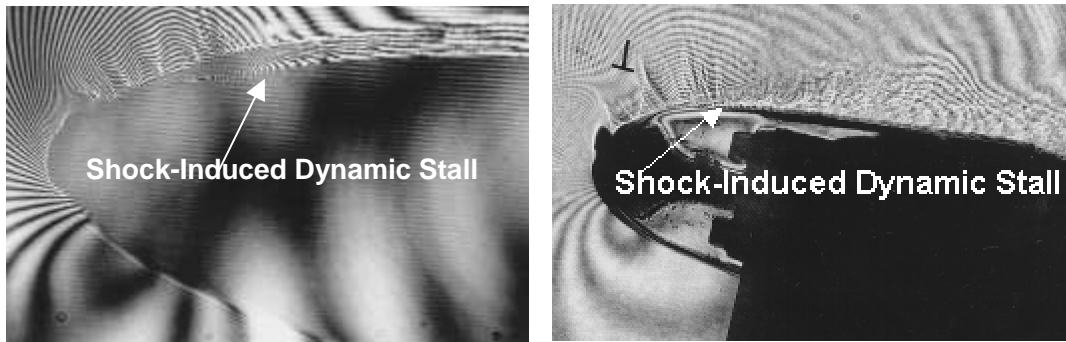
Fig.5. Comparison of flows over the NACA 0012 and the DDLE airfoils, M = 0.4 , k = 0.05 ; (a) \alpha = 10.5^\circ , (b) \alpha = 13^\circ , Shape = 3.5
