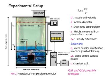
Figure 1: The apparatus for simulation of cumulus cloud flows.
