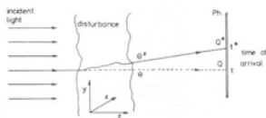
Fig. 1 Deflection and retardation of a light ray in an optical disturbance.
